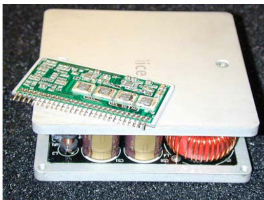
Figure 23 Comparing 250W/8Ω AT core (Substrate on top) with 250W/8Ω PMA module (ICEpower500A size 4”x 4” x 1”)
